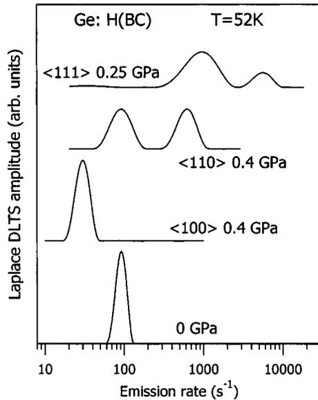
FIG. 26. Reproduced from Dobaczewski *et al.* (Ref. 78). Demonstration of the trigonal symmetry of bond-center hydrogen in Germanium from the splitting of emission peaks under uniaxial stress applied along  $\langle 100 \rangle$ ,  $\langle 110 \rangle$  and  $\langle 111 \rangle$  crystal directions.
