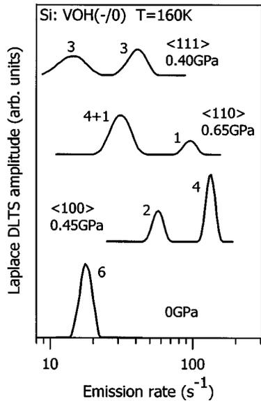
FIG. 35. Reproduced from Coutinho *et al.* (Ref. 130). Laplace DLTS spectra of VOH(-/0) recorded at 160 K at zero stress and under uniaxial stress along the three major crystallographic directions. The splitting pattern establishes the effective (i.e., thermally averaged) orthorhombic- $I$  ( $C_{2v}$ ) symmetry of (cf. Fig. 30).
