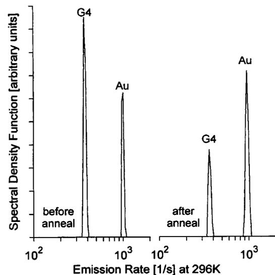
FIG. 5. Reproduced from Deixler *et al.* (Ref. 37 ). Comparison of Laplace spectra of the G4 and gold-acceptor level taken (left) and after (right) annealing at 250 °C for 5 min. The results of the two measurement are presented on the same scale. It can be seen that the G4 peak is reduced substantially while the gold-acceptor peak shows a small increase.
