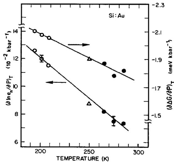
FIG. 22. Reproduced from Samara and Barnes (Ref. 60). Temperature dependence of the logarithmic pressure derivative of the emission rate and the pressure derivative of the Gibbs free energy  $\Delta G$  needed to emit an electron from the Au acceptor level in silicon. When corrected for the contribution from the band edge (cf. Fig. 21) the isothermal pressure derivative of  $\Delta G$  measures the breathing mode lattice relaxation of the defect which accompanies the emission.
