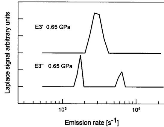
FIG. 27. Reproduced from Bonde Nielsen *et al.* (Ref. 122). Laplace spectra obtained under  $\langle 100 \rangle$  stress to demonstrate the lowering of the trigonal symmetry of bond-center hydrogen in silicon (the  $E3'$  signal). After the conversion  $E3'$  to  $E3''$  by annealing the emission peak splits in the ratio 2:1 corresponding to monoclinic symmetry.
