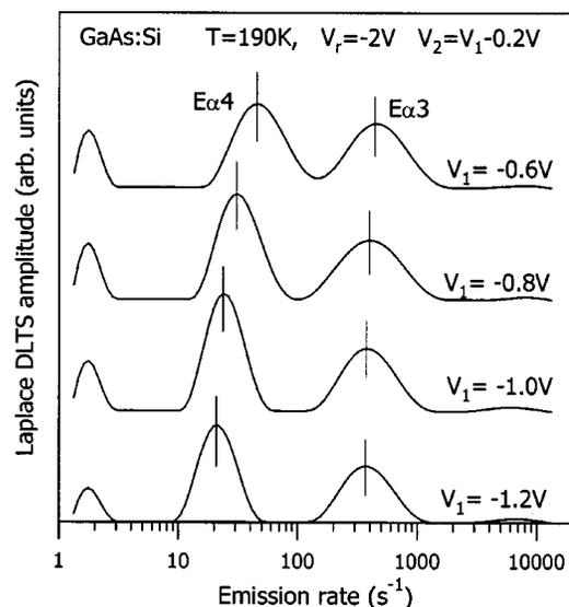
FIG. 17. A series of the Laplace DLTS spectra taken at different electric fields (in the differential mode) for the  $\alpha$ -particle irradiated sample of GaAs:Si. The electric field (it is the lowest for the bottom spectrum) increases the emission rate for the E $\alpha$ 4 defect, while for the E $\alpha$ 3 defect the effect is very weak (Ref. 73).
