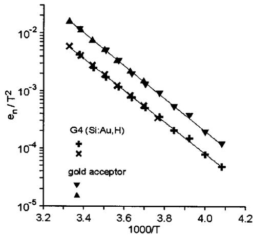
FIG. 6. Reproduced from Deixler *et al.* (Ref. 37). Arrhenius plots, obtained DLTS measurements, of the thermal emission rates for the gold-hydrogen level G4 and the gold-acceptor level. The different symbols on each line represent measurements taken in different laboratories on different samples. Activation energies derived from the slope of the least mean square fit are 542 meV (G4) and 558 meV (gold acceptor).
