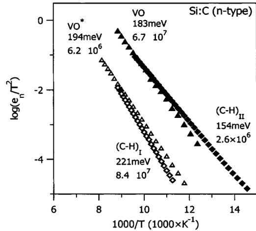
FIG. 9. Arrhenius plots of the  $(C-H)_I$ ,  $(C-H)_{II}$ ,  $VO^*$ , and VO defects measured at exactly the same experimental conditions. The plots demonstrate differences between the emission characteristics of the carbon- (square) and oxygen-related defects (triangles) in the stable (full symbols) and metastable (open symbols) configurations.
