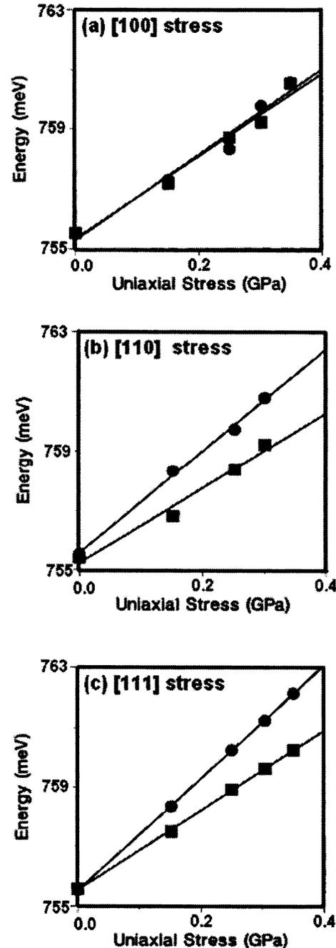
FIG. 25. Reproduced from Yang and Lamp (Ref. 117), the first reported attempt to maximize the separation of emission-rate signals in uniaxial-stress DLTS. The orientational splitting of the EL2( $0/+$ ) level is resolved by least-squares decomposition of digitized capacitance transients. The revealed split patterns comply with the  $C_{3v}$  symmetry expected for an axial interstitial pair  $As_{Ga}-As_i$ .
