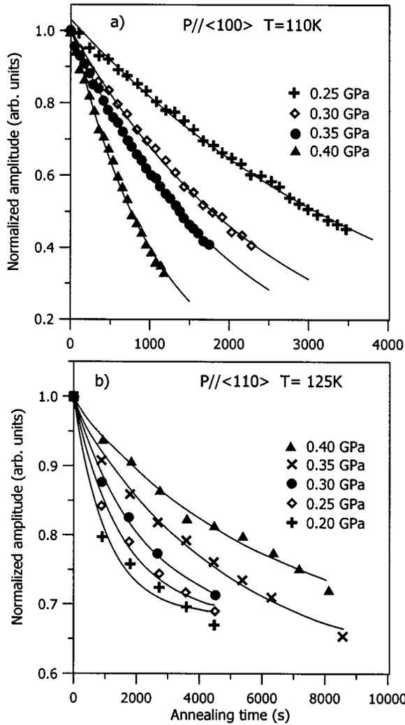
FIG. 33. Reproduced from Dobaczewski *et al.* (Ref. 88). The VO<sup>0</sup> reorientation kinetics measured from the change in amplitude of the stress-split Laplace DLTS peaks of Fig. 29 in a sequence of isochronal annealing steps at a fixed temperature. For <100> the reorientation time constant decreases with stress whereas for <110> the time constant increases with stress.
