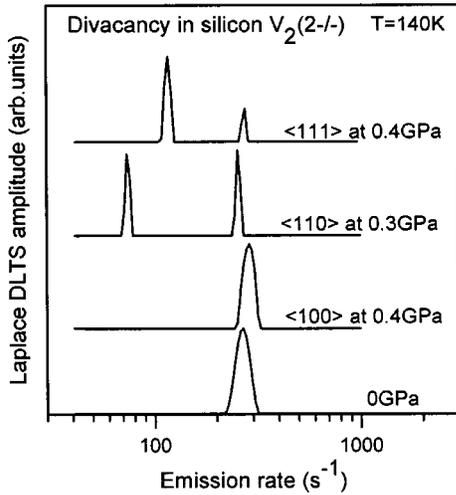
FIG. 37. Laplace DLTS spectra of the  $V_2(2-/)$  level taken without stress and with stress applied along the three major crystallographic directions (Ref. 136). The  $\langle 110 \rangle$  splitting is larger than the  $\langle 111 \rangle$  splitting indicating an anomaly in the otherwise trigonal pattern.
