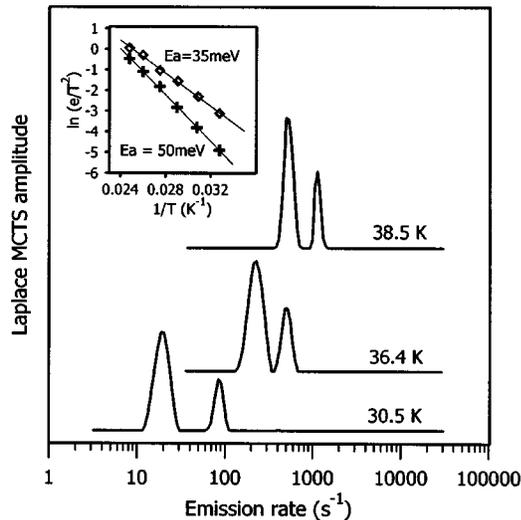
FIG. 12. Adapted from Gad and Evans-Feeman (Ref. 52). Laplace minority carrier transient spectra of hole emission from two point defects measured in *n*-type strained Si/Si<sub>0.855</sub>Ge<sub>0.145</sub>/Si quantum wells between 30.5 and 38.5 K. Arrhenius plots of the two states are shown in the inset.
