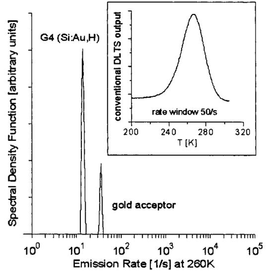
FIG. 4. Reproduced from Deixler *et al.* (Ref. 37) DLTS and LDLTS spectra of hydrogenated silicon containing gold. The conventional DLTS spectrum is shown as an inset at the top right of the figure. The broad peak centered at 260 K is attributed to electron emission from the gold acceptor and G4. The main spectrum uses the Laplace technique and clearly separates the gold-acceptor level and the gold-hydrogen level G4.
