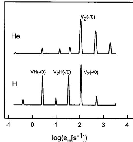
FIG. 7. Laplace DLTS obtained at 225 K. Lower plot, hydrogen-implanted sample ( $\sim 10^{10}$  cm $^{-2}$ ); upper plot, helium-implanted sample ( $\sim 10^9$  cm $^{-2}$ ). The samples have been implanted at 60 K and subsequently reverse-bias annealed at 400 K. (Ref. 44).
