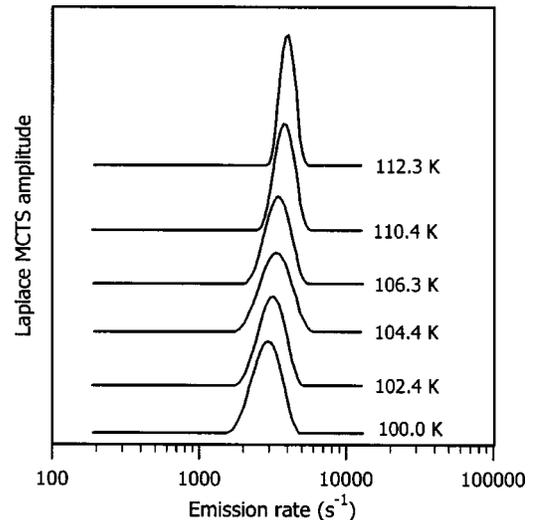
FIG. 13. Reproduced from Gad and Evans-Feeman (Ref. 52). The LMCTS spectra of thermally assisted hole tunneling from strained Si/Si<sub>0.855</sub>Ge<sub>0.145</sub>/Si quantum wells between 100 and 112.3 K.
