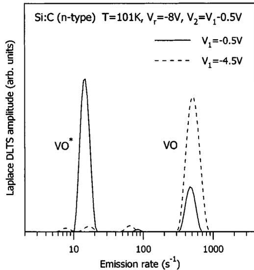
FIG. 8. The Laplace DLTS spectra taken in the differential mode for the silicon sample irradiated with electron at low temperature and measured *in situ*. The spectra show that the metastable configuration of the VO complex ( $VO^*$ ) is observed only close to the sample surface (solid line) due to the fact that at this region the annealing process of the defect occurs in the conditions of a low position of the Fermi level.
