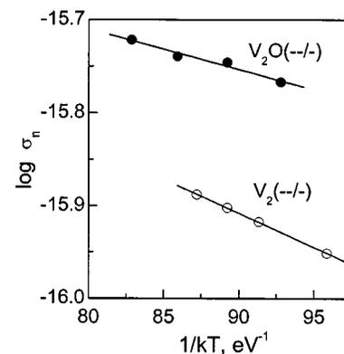
FIG. 11. Reproduced from Markevich *et al.* (Ref. 48). Temperature dependencies of electron capture cross sections for the double acceptor levels of the  $V_2$  and  $V_2O$  in silicon. Solid lines are calculated ones on the basis of the equation  $\sigma_n = \sigma_\infty \exp(-E_\sigma/kT)$  with parameters determined from least-square fits of experimental data.
