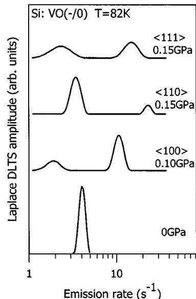
FIG. 29. Reproduced from Dobaczewski *et al.* (Ref. 88). Laplace spectra obtained for the orthorhombic-I VO center under uniaxial stress. Note that  $\langle 110 \rangle$  stress should cause splitting into three emission peaks with the intensity ratio 1:4:1. Only two with intensity ratio 5:1 is observed. The true splitting is revealed for stress  $>0.6$  GPa.
