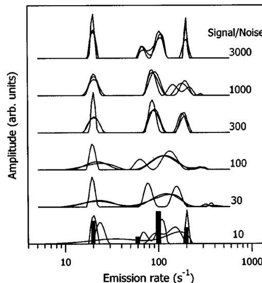
FIG. 2. Results of numerical tests demonstrating a role of the noise on the resolution of the methods implemented in the system described in this work. The bar diagram depicts the emission rates and amplitudes of four monoexponential components assumed in the simulated transients. For a given noise level three different numerical routines have been used.
