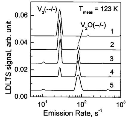
FIG. 10. Reproduced from Markevich *et al.* (Ref. 48). Development of Laplace DLTS spectra measured at 123 K for an electron-irradiated Cz-Si sample with an initial resistivity of 5  $\Omega$  cm upon 30 min isochronal annealing with temperature increments of 25°C. The spectra were measured after anneals at (1) 150, (2) 200, (3) 225, (4) 250, and (5) 275°C. Measurement setting were bias  $-5 \rightarrow -0.2$  V and pulse duration 1 ms.
