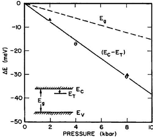
FIG. 19. Reproduced from Samara (Ref. 86). Hydrostatic pressure dependence of the activation energy  $E_C - E_T$  (or  $\Delta H$ ) for the vacancy-oxygen center VO in silicon compared with that of the energy gap  $E_g$ . The insert depicts the fact that the VO level moves closer to the conduction band (and farther from the valence band) with pressure. From the graphs it can be deduced that  $E_T$  moves away from the valence-band edge at a rate of 24 meV/GPa.
