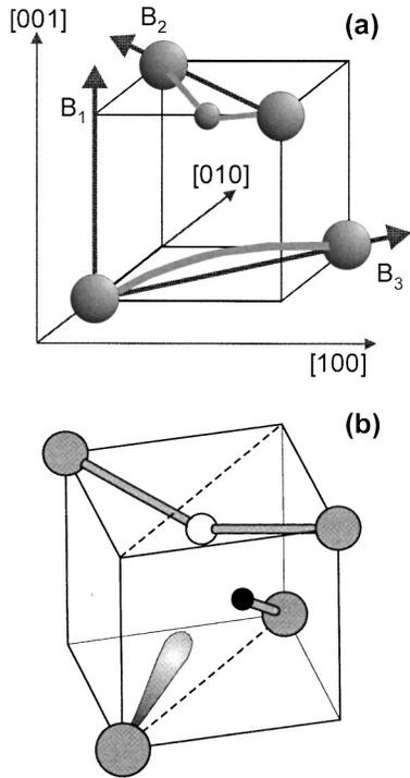
FIG. 30. (a) The geometric structure of the VO defect. The arrows indicate the principal axes of an orthorhombic-I piezospectroscopic tensor. The labels  $B_1$ ,  $B_2$ ,  $B_3$  denote the corresponding eigenvalues. (b) The modification of the structure (a) when VO traps a hydrogen atom.
