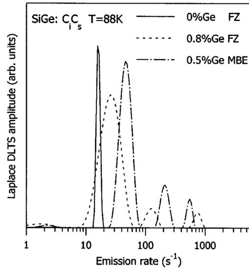
FIG. 16. The Laplace DLTS spectra of the  $C_i-C_s$  pair observed in the FZ silicon (solid line), FZ SiGe (0.8% of Ge) (dashed line), and the MBE-grown strained SiGe (0.5% of Ge) (dotted-dashed line) samples (Ref. 62).
