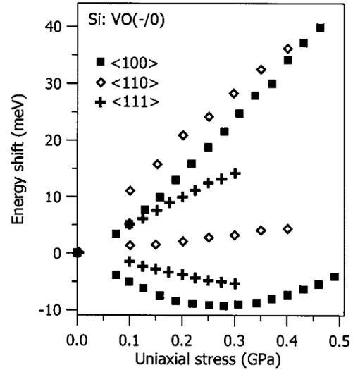
FIG. 31. The stress dependence of VO for the three major stress directions  $\langle 100 \rangle$ ,  $\langle 110 \rangle$  and  $\langle 111 \rangle$  defined as  $\Delta E = k_B T \times \ln[e_n(P)/e_n(P=0)]$ , from Dobaczewski *et al.* (Ref. 88).
